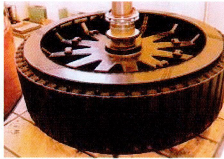
Rotor of synchronous generator
