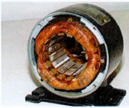
Main parts of induction motor: 1. stator
