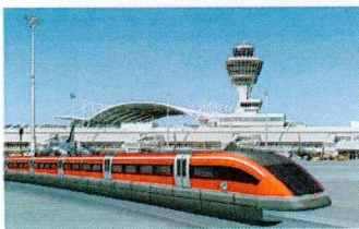
Linear induction motors are used in this Maglev rapid transportation
