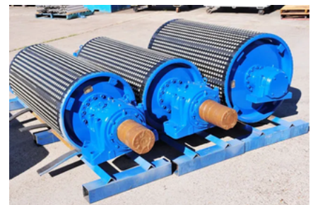
Conveyor Drive Pulley
