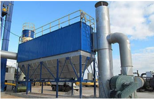
Dry Dedusting System
