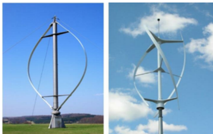
Vertical Axis Wind Turbine
