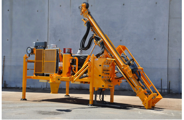
Air Core Drill Rig
