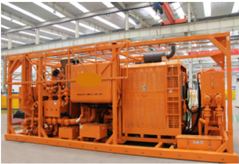
Single Pump Cementing Unit
