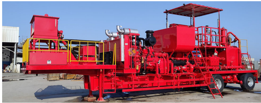
Twin Pump Cementing Unit
