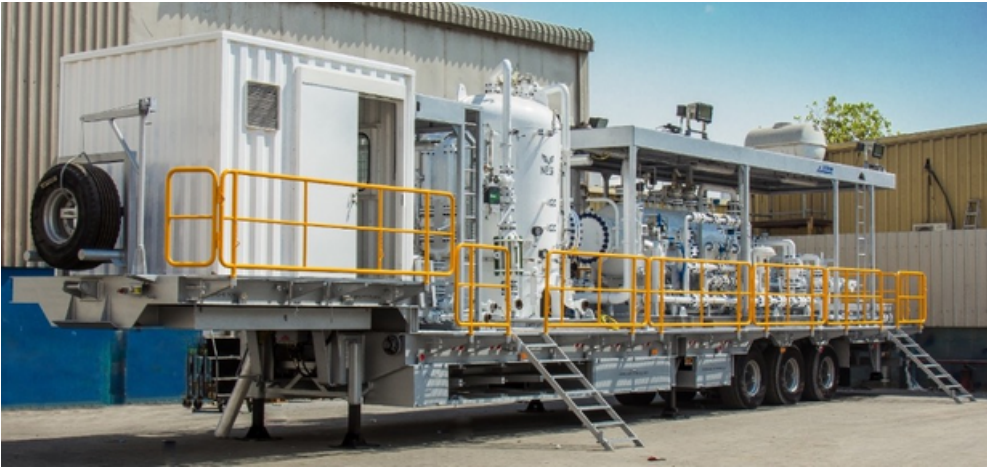
Trailer Mounted Well Test Equipment
