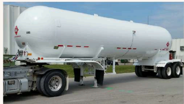
High pressure tank
