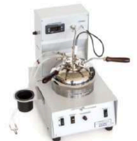
Flash point by Tag Closed Tester
