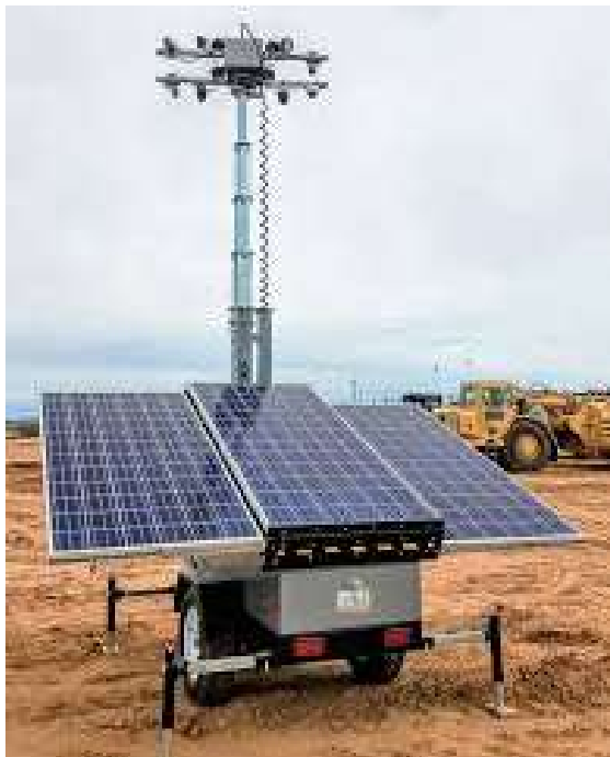
Solar Lighting set
