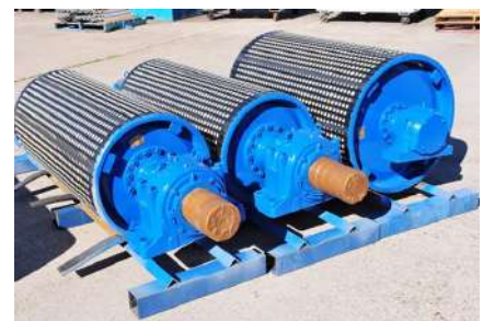
Conveyor Drive Pulley
