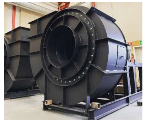
Gas Flow Fans
