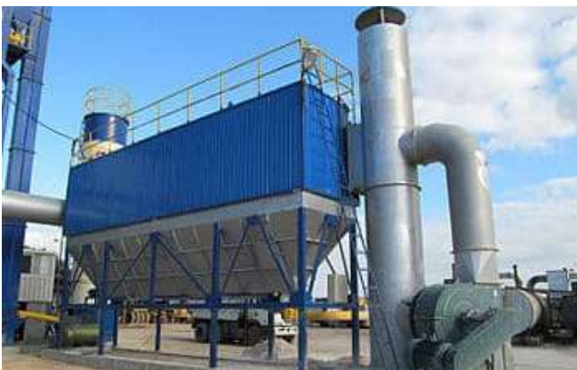
Dry Dedusting System
