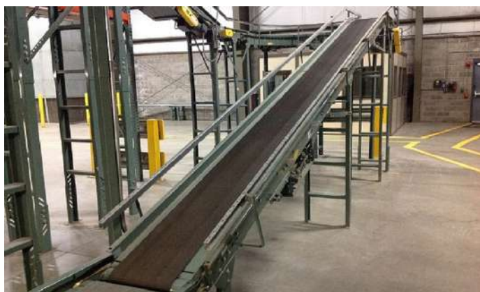
Belt Conveyor system
