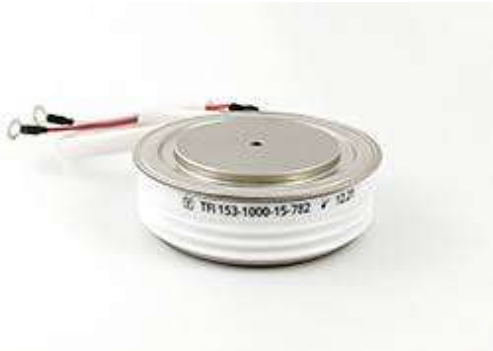
Fast-switching thyristors or SCRs
