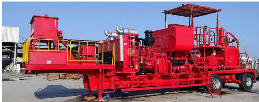
Twin Pump Cementing Unit
