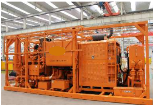
Single Pump Cementing Unit
