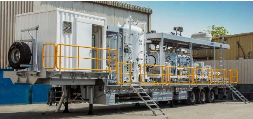
Trailer Mounted Well Test Equipment
