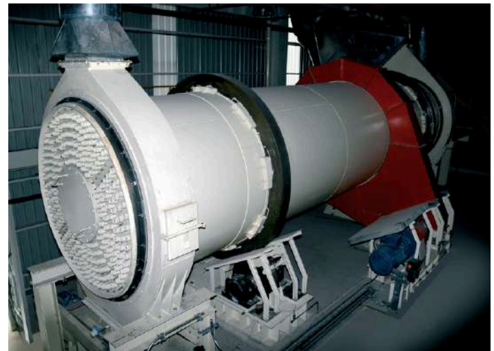
Rotary Drum Cooler for Calcined Gypsum
