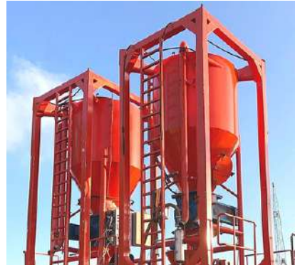
Cement Surge Tank
