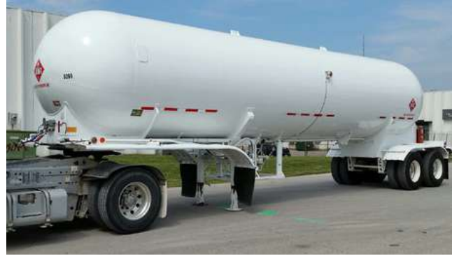
High pressure tank
